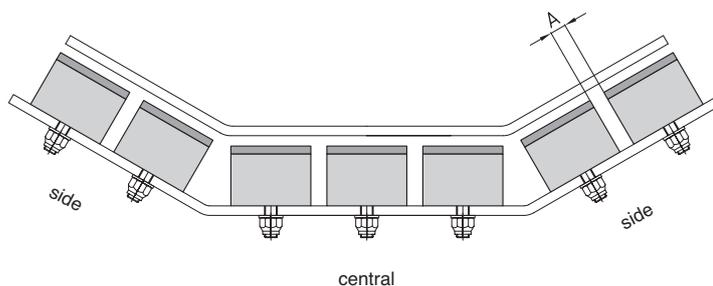
To be used for transoms with 20°- 30°- 35° inclination angle.
