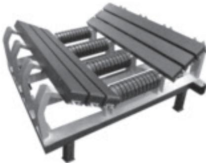
Rulmeca presents a new product to widen the range of components for belt conveyors: impact bars used at the loading point of the conveyor under the hopper. These impact bars utilise the important properties of two materials such as the low friction of polyethylene and a quality rubber to absorb shocks.
