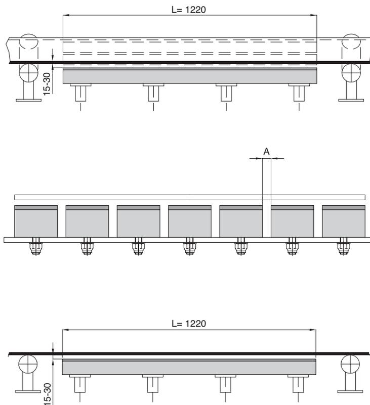
Impact bars must be installed to keep the clearance distance from the under-side of the belt to 15 mm for light applications and 30 mm for heavy applications.
