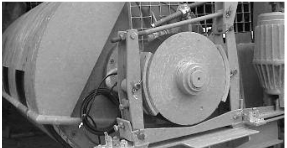
Both Motorized Pulleys are fitted with brake shaft for connection to external brakes.
